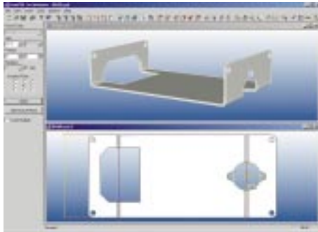
The associativity between 3D model and 2D flat pattern allows simultaneous work in both modes.
