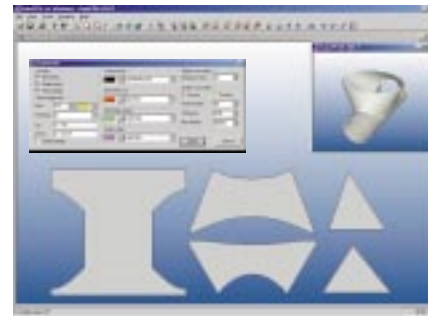
Configurable output when exporting unfolded geometry as DXF files. Line types and colours can be selected. Bend angles can be included.
